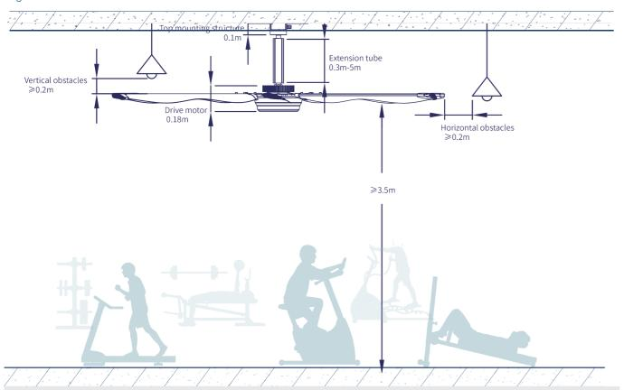
NOTE: be cautious of items like light fittings which may swing into the path of the spinning fan, ensure appropriate clearance is maintained.
